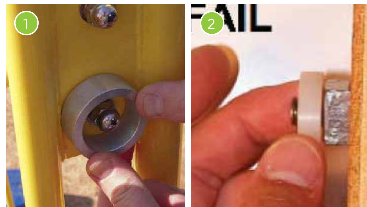
Gauges are used to test the compliance of all projections. This projection is in compliance because it does not extend beyond the face of the gauge.
