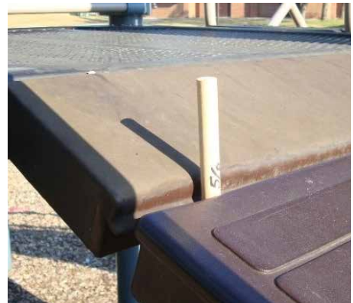
Demonstration of test for crush and shear hazard.
