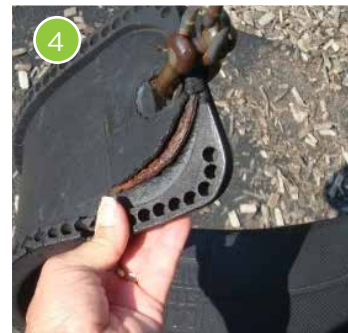
This belt swing is tearing and should be replaced.
