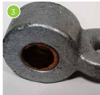
This bushing (red) is worn and should be replaced.
