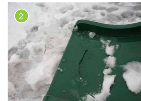
This tear could be an entanglement hazard.
